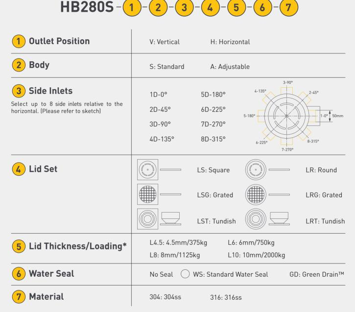
\*Lid Loading is a conservative figure arrived at by solids analysis and refers to a point load. A spread load will translate to a higher load carrying capacity by the lid.
